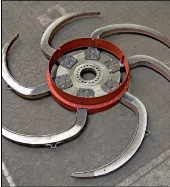
Single Discharge Wheel with six arms
