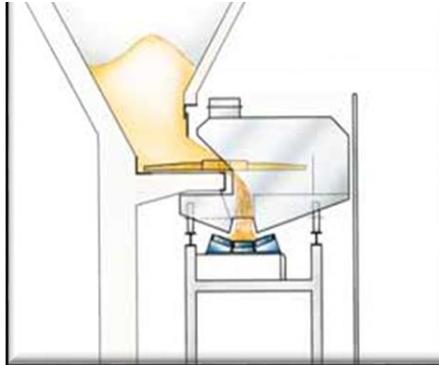
RDM with double swivel drive for single side discharge on both sides
